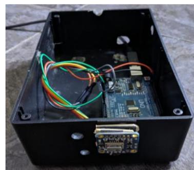
**Gambar 27.** Rangkaian Sensor Suhu amg8833
