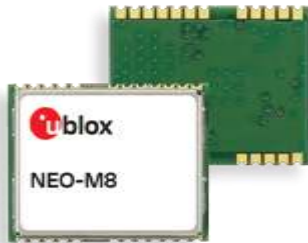
Gambar 1 Penerima GNSS komersil (u-blox.com/en/product/neo-m8-series)
