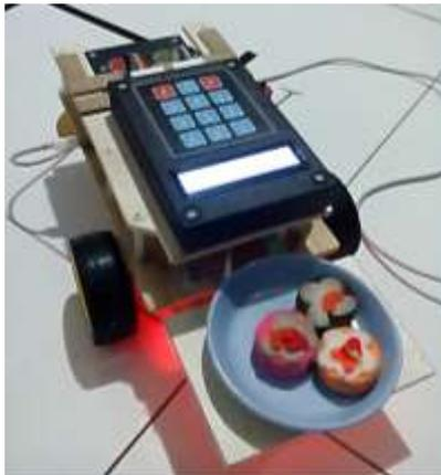
**Gambar 10.** Rancangan Prototype Robot Pelayan
