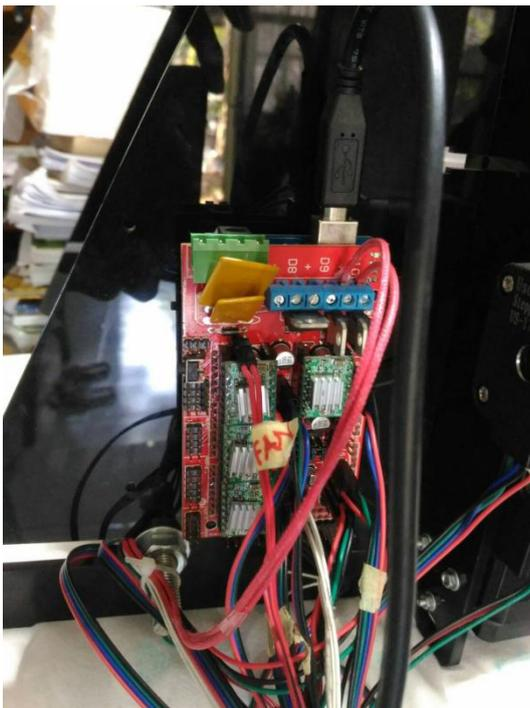
Gambar 5 Arduino mega + shield (hardware)
