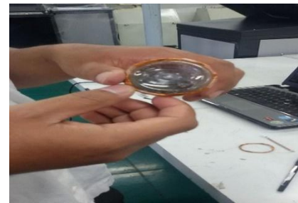
Gambar 11. Proses Melilit Antena
