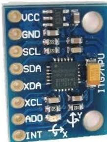
**Gambar 1.** Sensor MPU 6050 – 3 axis *accelerometer* + 3 axis *gyroscope*
