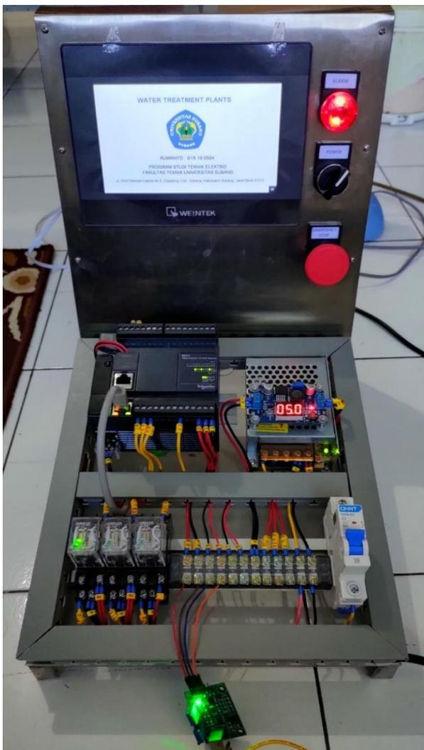
**Gambar 19** Prototipe SCADA Koagulasi
