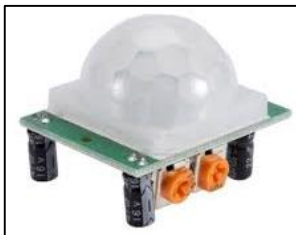
Gambar 1. Sensor PIR HC-SR501
