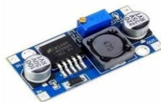
Gambar 11. Modul Step Down DC-DC[20]
