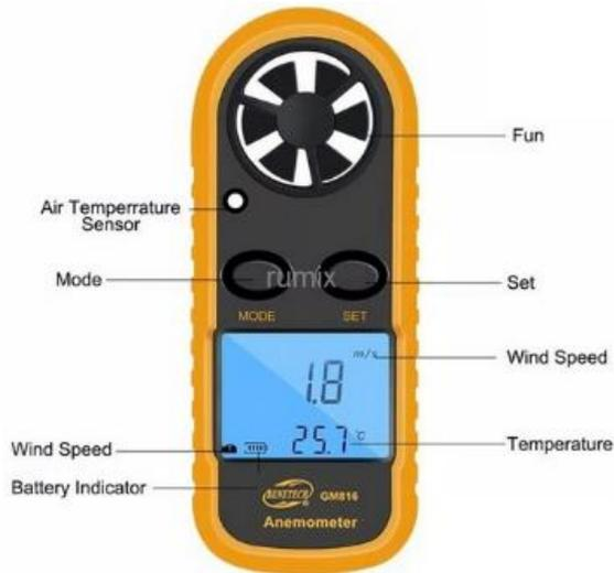
Gambar 5. Anemometer Digital
