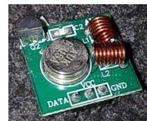
Gambar 11. Modulator TX-FST3
