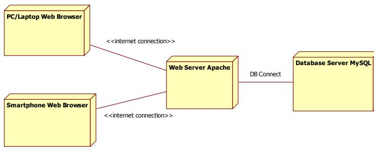
Gambar 4.11 Deployment Diagram
