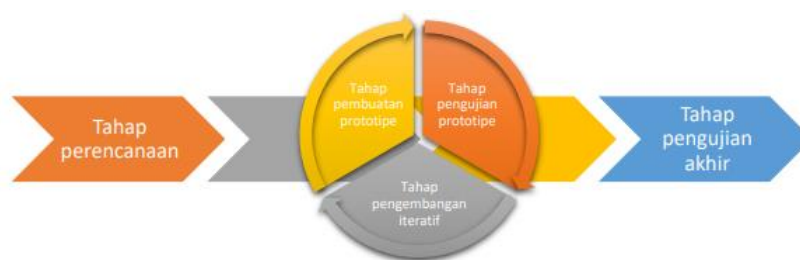
Gambar 1. Rapid Application Development (RAD) dengan metode prototyping [6]
