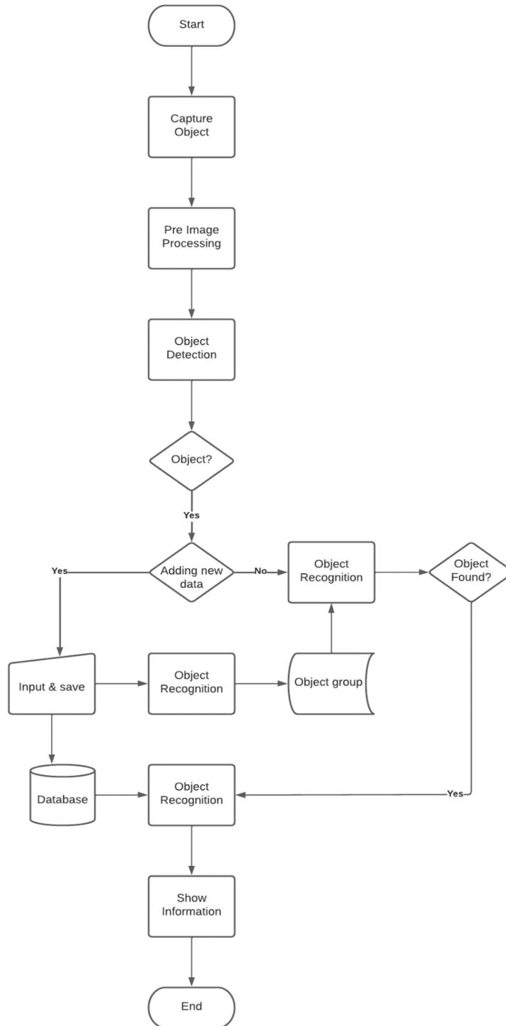
**Figure 1.** Identify the object using the Eigenface PCA method
