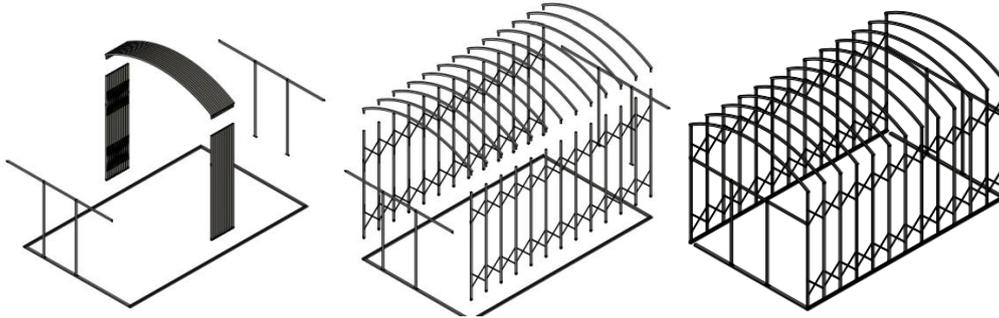
**Figure 8.** Foundation Frame and Mushroom House Frame Assembly
