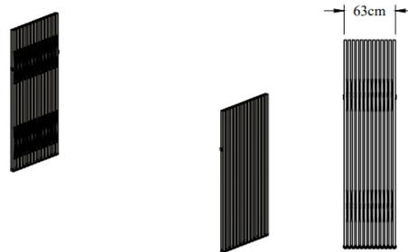
**Figure 5.** The Left and Right Wall Frames Are Closed Together
