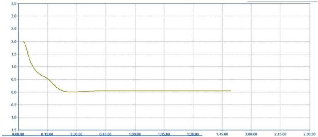
**Figure 3.** Graphic obtained from the Guarded Hot Plate Test for Stacked TetraPak Packages (time x thermal conductivity)
