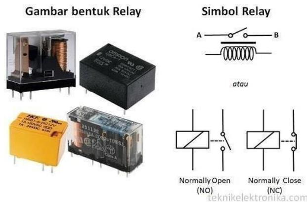
Figure 3. Relayed shape module
