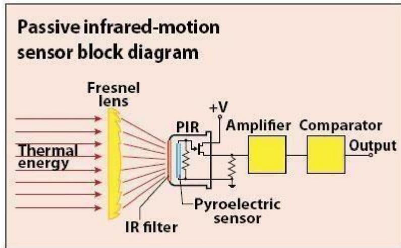
**Figure 1.** PIR sensor movement diagram
