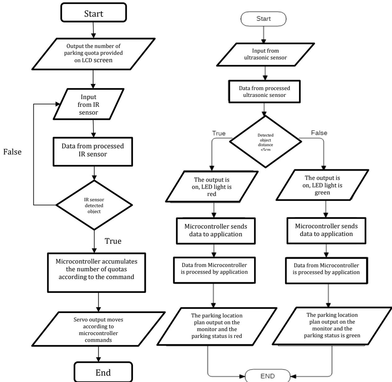
Figure 4. a. Flowchart Parking Quota View b. Flowchart Parking Location View
