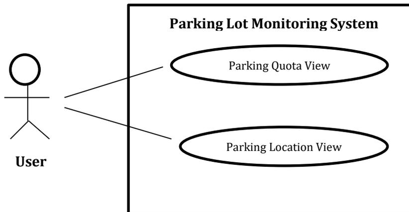
Figure 2. Usecase Diagram of Parking Lot Monitoring System
