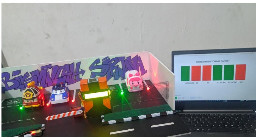
**Figure 6** Partially Filled Slot Implementation View
