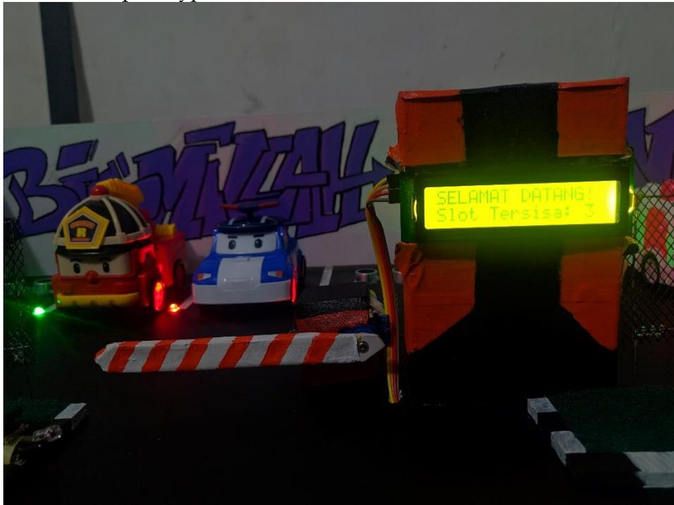
**Figure 5** Parking Quota on LCD Display
