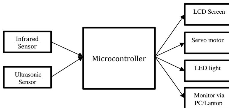
Figure 3. Block Diagram of Parking Lot Monitoring System
