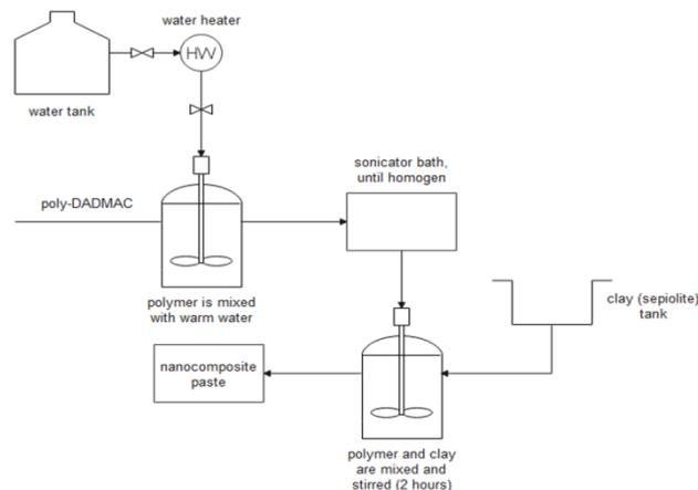
**Figure 1.** Process Flow Diagram (PFD) for production of nanocomposite from poly-DADMAC and sepiolite
