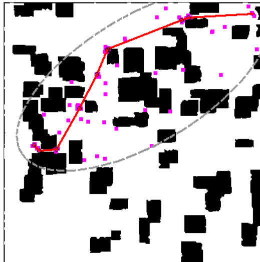
Figure 7. The path with the lowest solution cost generated by the EI-PRM algorithm in the BIT* clutter map
