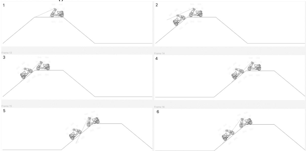
**Figure 8.** The tool will adjust the angle of inclination when the motorcycle wants to pass through the descent
