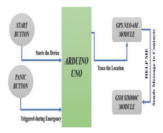
Fig. 7. Diagrammatic view of tracking and sending location
