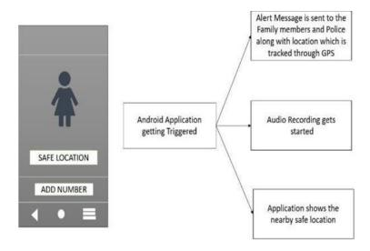
Fig. 5. Additional Features supported through Android Application
