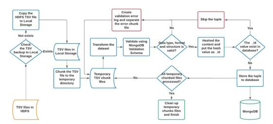
Fig. 10. XBRL Dataset Loader Feature Diagram
