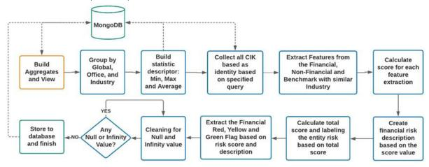
Fig. 14. XBRL Analyzer and AI Features-Extraction feature
