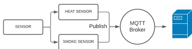
**Fig. 5. MQTT Publisher-Broker Architecture**
