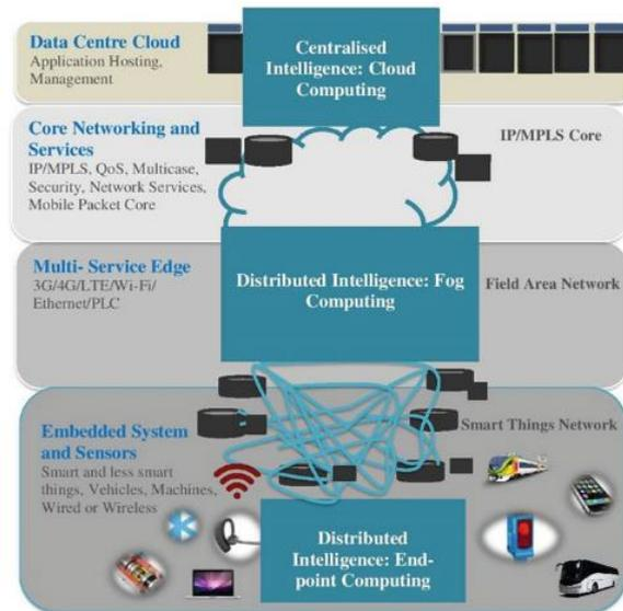
Fig. 2. Fog Computer Architecture (Zhu *et al.*, 2013)
