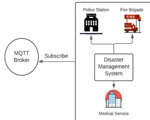
**Fig. 6. MQTT Subscriber-Broker Architecture**
