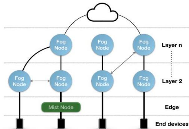
Fig. 4. Fog Computing Architecture (Battistoni *et al.*, 2019).
