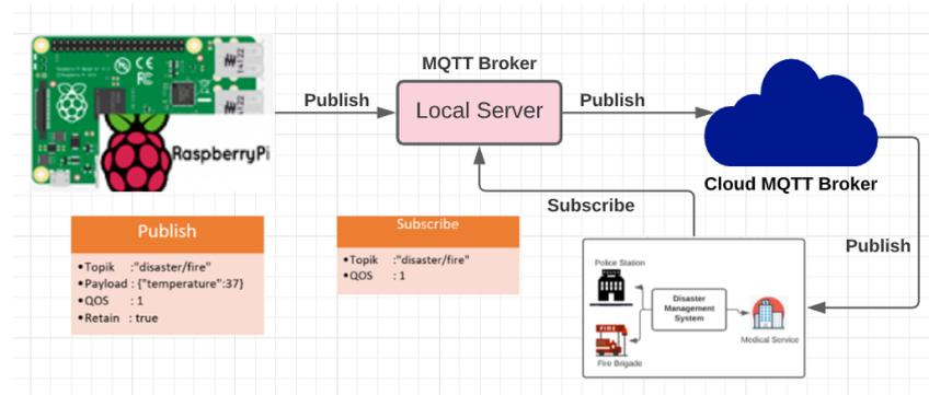
**Fig. 7. MQTT Connection of the IoT, Fog and the Cloud**
