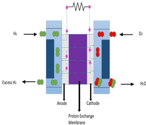
**Fig. 1 Diagram for illustration of PEMFC**
