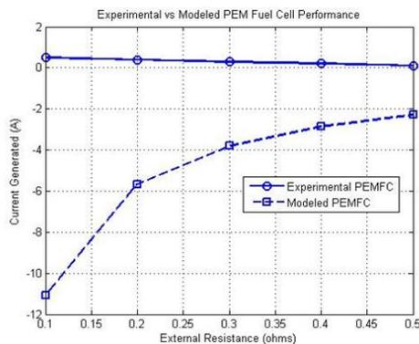
Fig. 5. Experimental vs modeled PEMFC's performance
