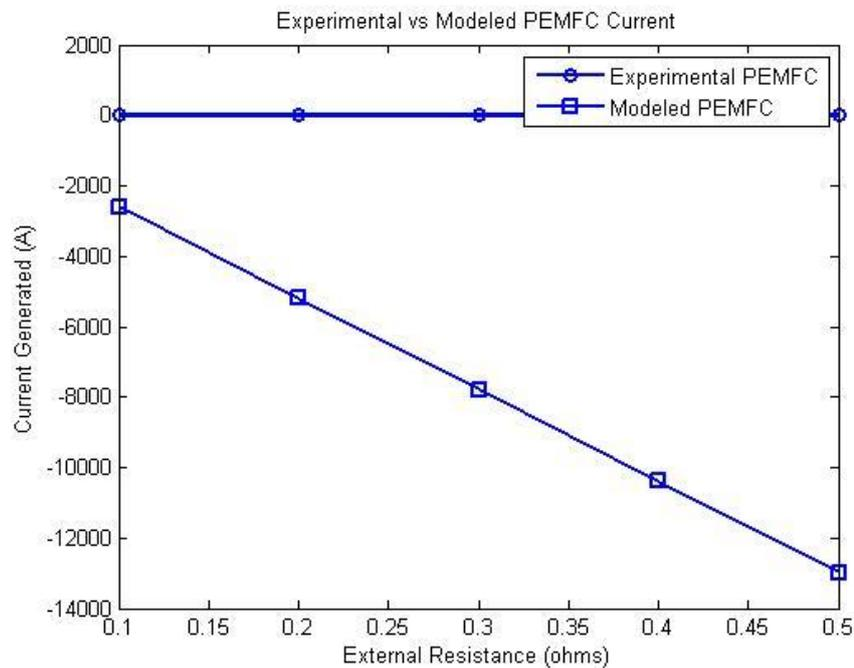
**Fig. 9. Plot for resulting current variation in experimental and modeled PEMFC**
