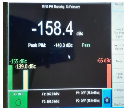
Fig. 9. Frequency-domain trace PIM level for 850MHz band - Pass scenario @25dBm RF power
