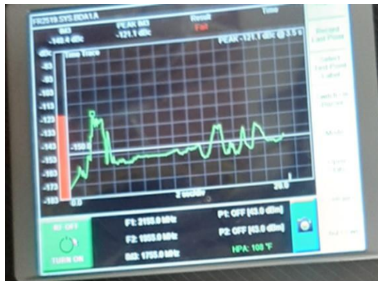
Fig. 7. Time- domain trace PIM signal level versus time – Fail scenario @43dBm RF power for band 4
