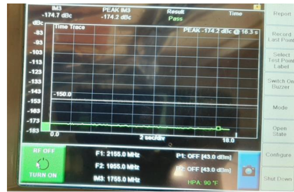
Fig. 3. Time domain trace PIM signal level versus time Pass scenario @43dBm RF power for band 4
