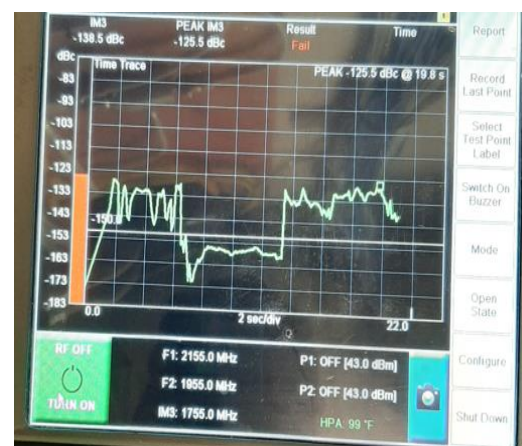
Fig. 5. Time- domain trace PIM signal level versus time - Fail scenario @43dBm RF power for band 4
