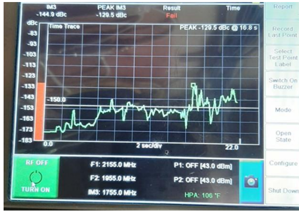
Fig. 6. Time- domain trace PIM signal level versus time – Stress test scenario @43dBm RF power for band 4
