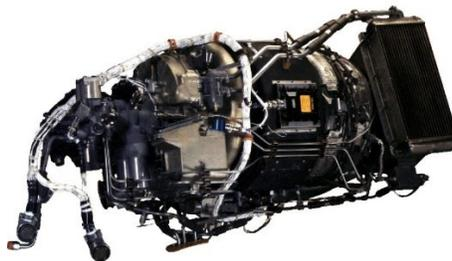
**Gambar 1. APU (*Auxiliary Power Unit*)**
