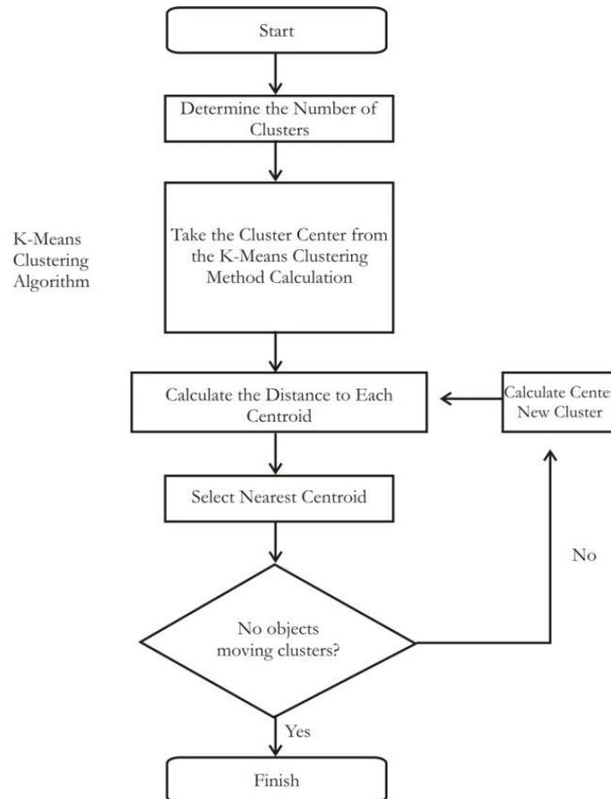
Figure 3. K-means Algorithm Flowchart
